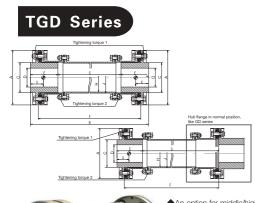
An option for middle/high speed applications Hubs in an inversion form, small additional bending moment, especially suitable for turbinecompressors sets
